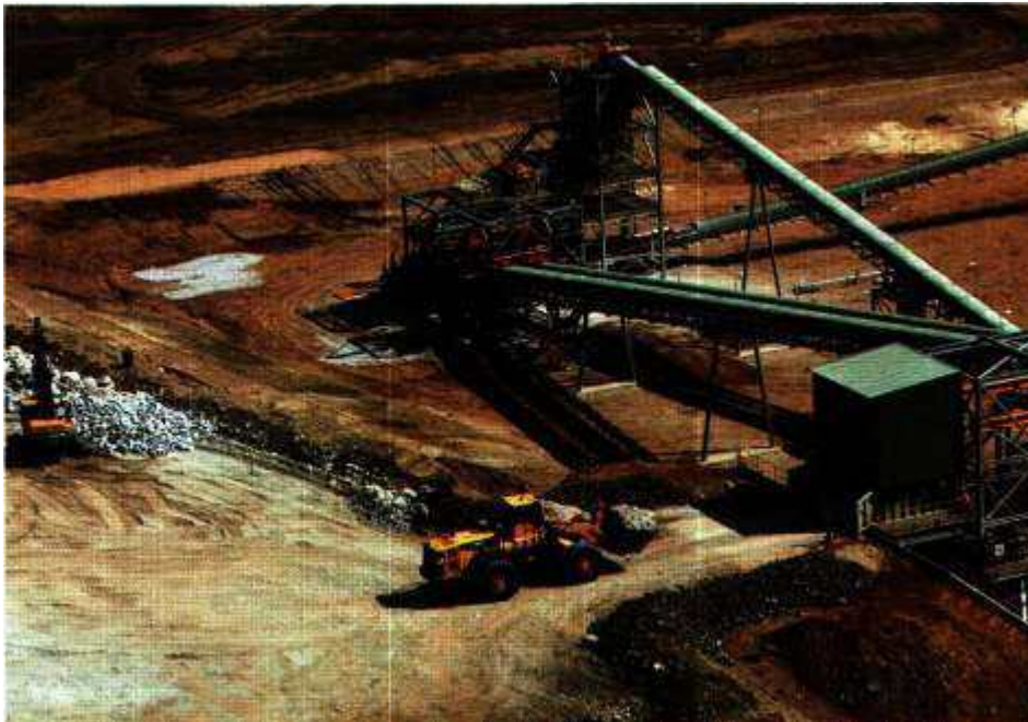
Mt Cattlin ore being loaded into the crusher.
